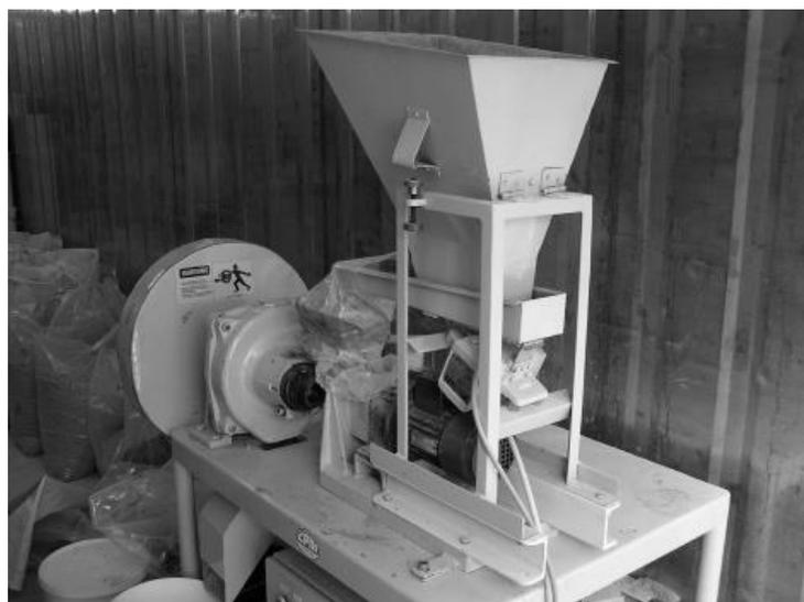
Figure 3 : Bench-scale California pellet mill at DTU [2].
