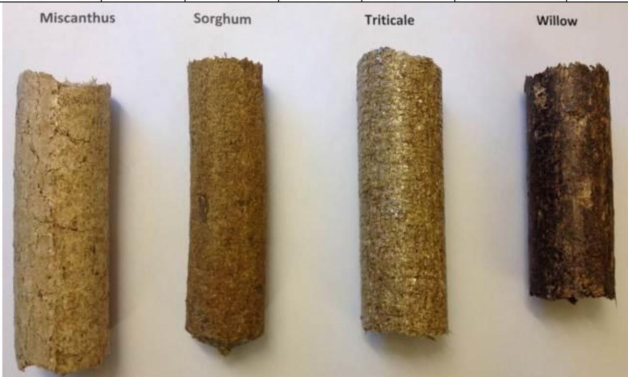
Figure 14 Briquette samples from the trial runs
