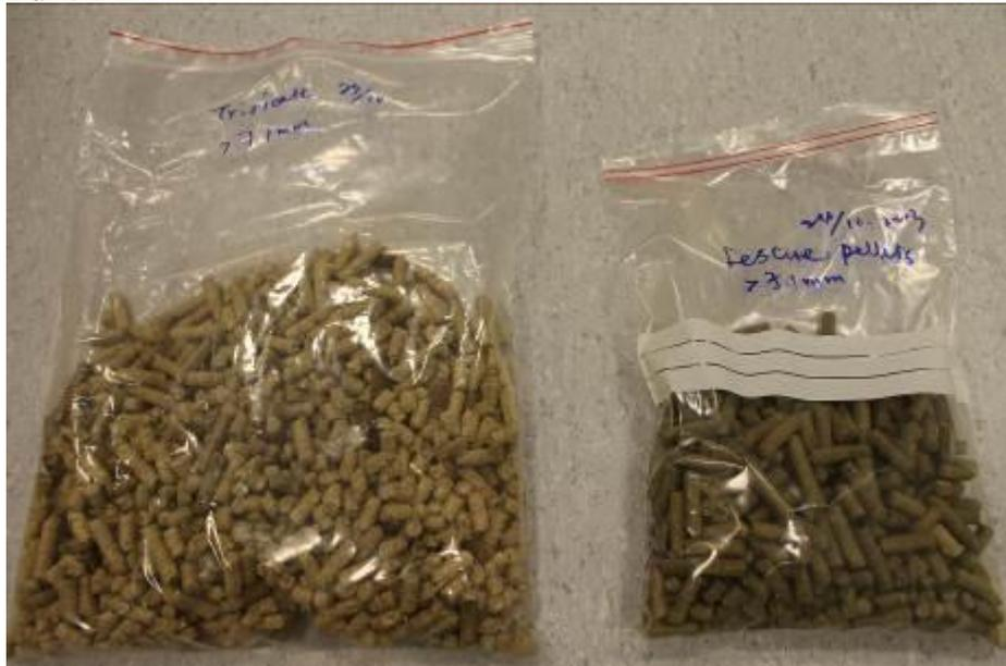
**Figure 8 : Triticale pellets (left) and fescue pellets (right) from the bench-scale pelletizer.**
