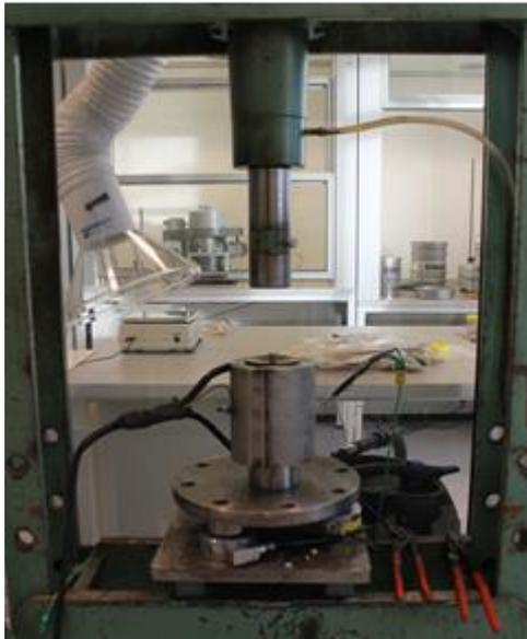
Figure 1 : Picture of single-pellet press
