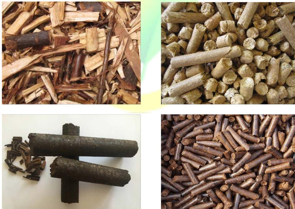
Figure 3 Untreated *Willow* and torrefied *Willow* briquettes (left) and pre-pelleted *Triticale* and torrefied *Triticale* pellets (right)
