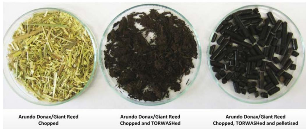
Figure 2 Untreated, torwashed and pelletised *Arundo Donax* Giant Reed
