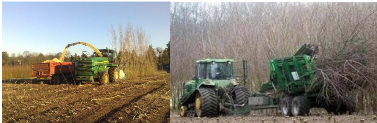
FIGURE 1. A SELF-PROPELLED FORAGE HARVESTER FITTED WITH A SRC CUTTING HEADER (COPPIC RESOURCES LTD) PRODUCING WOOD CHIPS (LEFT) AND A TRAILED STEMSTER III (NORDIC BIOMASS) CUTTING WHOLE RODS (RIGHT).
