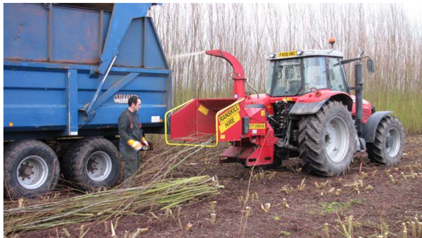
FIGURE 2. CHIPPING RODS WITH A FORESTRY / ARBORICULTURAL CHIPPER.
